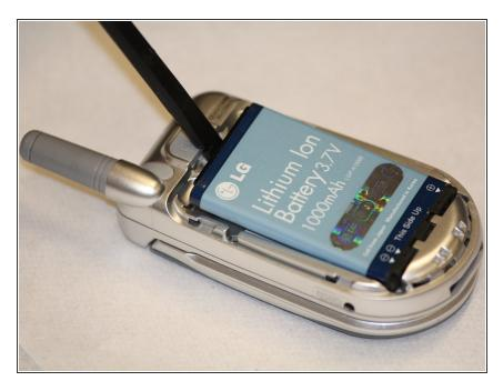
From the lip on the top of the battery, lift it out of the phone.
