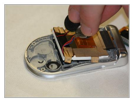
To remove the screen, grab hold of one or more of the speakers and pry up using the connecting wire. The tape holding the screen in should lift up, and the screen should easily separate from the case.
