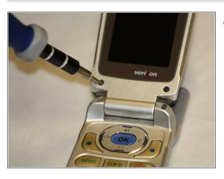
Remove the four screws using your Phillips head screwdriver.
