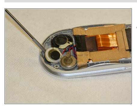
The speakers are held in by a sticky glue. Be careful not to break any of the components, simply pry slowly from underneath until the speakers pop out.
