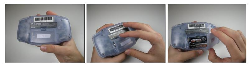
• Remove the back battery cover by pinching down on the tab and pulling outward.
