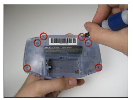
Remove the six back panel screws using a Y1 screw driver.
