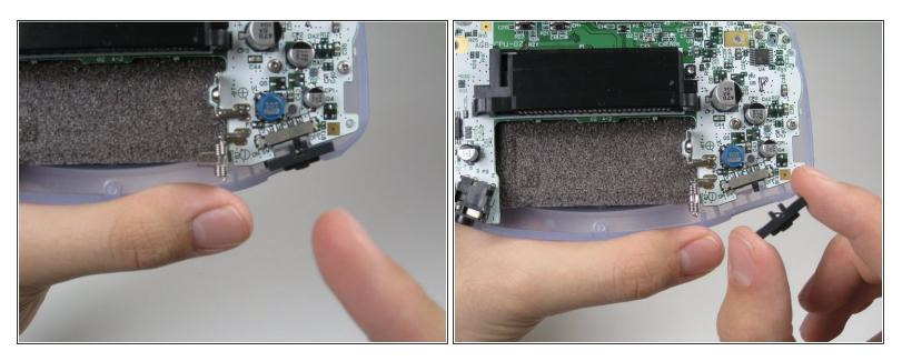
Remove the gray On/Off Switch by pulling up and away from the unit. Replace with another switch if necessary.
