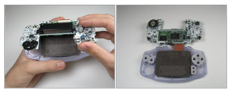
• Pull circuit board away from the front panel by pulling up at the bottom of the circuit board, keeping the top ribbon still connected.
