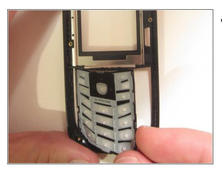
• Rotate and remove the keypad from the front case.
