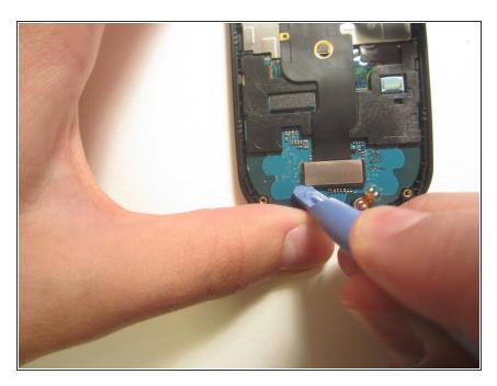
• Detach the ribbon cable with the plastic opener.
