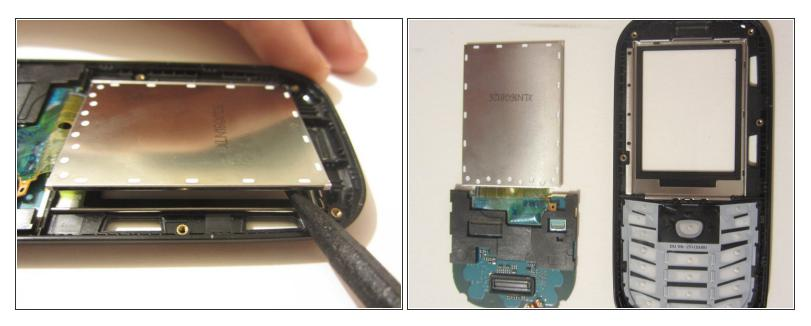
Use a tool to pry open the LCD display. Remove the display and the motherboard-looking device that it's connected to.
