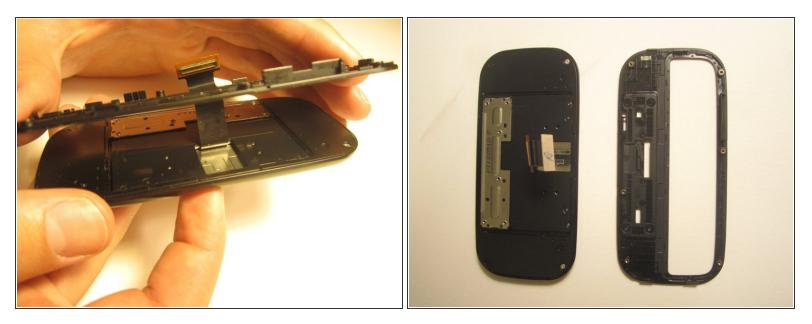
• Pull the ribbon cable through the slit in the keyboard case to separate it from the sliding mechanism.
