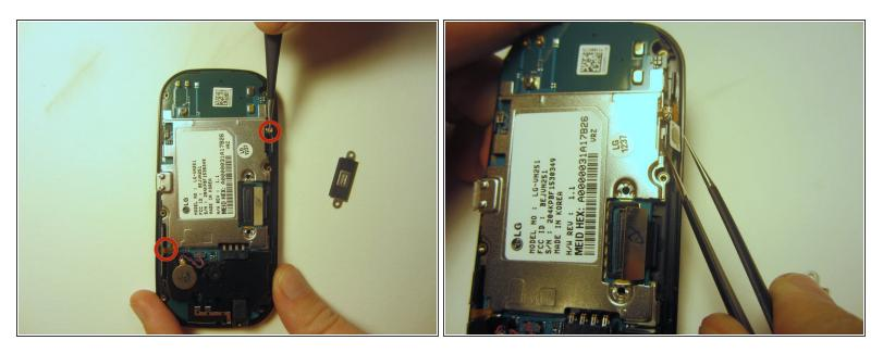
Use tweezers to disconnect the two cables that attach the motherboard to the case.
