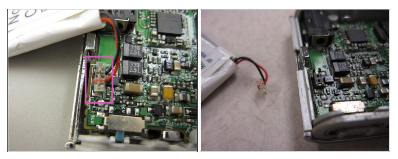
• Unplug the battery connecting cables.
