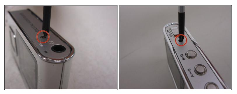
Remove the screw on each side of the device using a Phillips head screwdriver.
