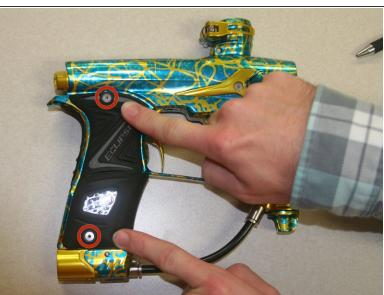
Remove the four screws from the grip with the 5/64" allen wrench. There are two on each side.
