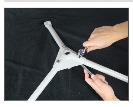
Tighten each nut using two 14mm wrenches until each leg is stable and the tripod will stand on its own. To disassemble your device, follow these instructions in reverse order.
