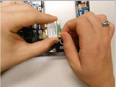
Disconnect the wires on the WiFi card. This can be done easily by applying pressure to the connections until they pop off of the card.
