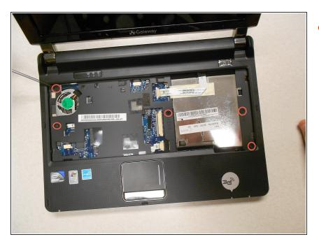
Remove the five (5) 5mm screws shown here using the Phillips #0 screwdriver.
