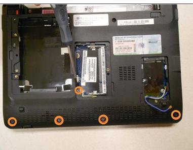
Remove six (6) 5mm screws, two (2) 17.5mm screws, and three (3) 2.5mm screws from the back, using the Phillips #0 screwdriver, as marked here.
