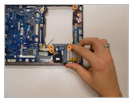
Using a Phillips #00 screwdriver, remove the four (4) 5mm screws holding the motherboard in place.
