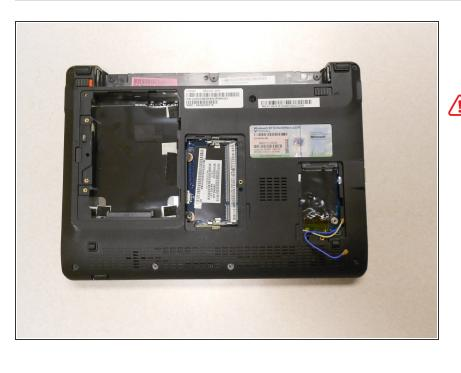
Make sure the RAM, hard drive, and WiFi card have been removed from the computer before trying to take off the cover so they are not damaged in the process.
