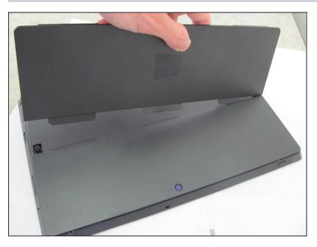
To remove the kickstand, gently pull up until the three tabs slide out of the slots on the back of the device.
