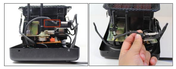
(i) Make note of where you disconnect the wires from so you can properly connect them when re-assembling heater.
