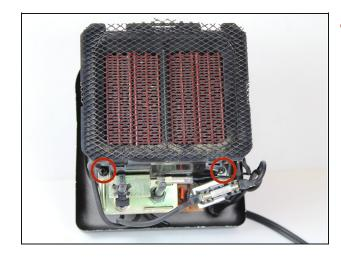
• Remove the two 10 mm Phillips screws using a #2 Phillips screw driver. One attaches the gold metal bracket to the heater coil housing and the other attaches the fuse holder to heater coil housing.
