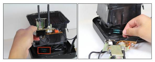
(i) Make note of where you disconnect the wires from so you can properly connect them when re-assembling heater.
