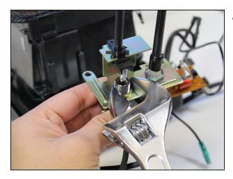
• Use an adjustable wrench to loosen the nut holding the switch to the metal bracket. Place the wrench around the nut and turn it counterclockwise.
