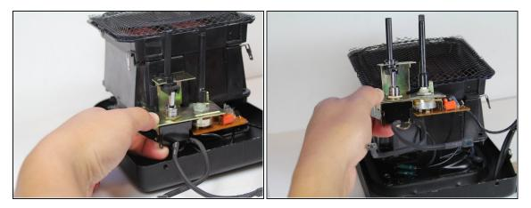
• Grab the Switch and Circuit Board Assembly with one hand and slide it up. You will need to wiggle it to break it loose. While wiggling it, slide it up until it is clear of the plastic rails.
