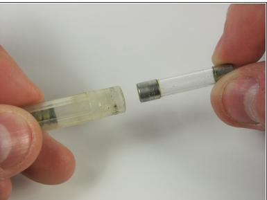
Remove the fuse from the case.
