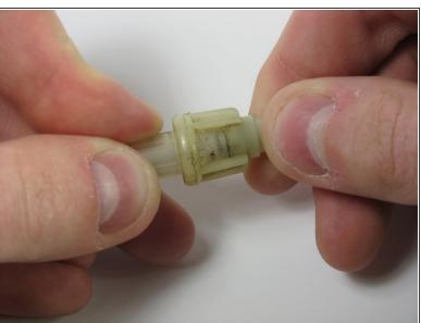
Simultaneously push the fuse container together and rotate counterclockwise.
