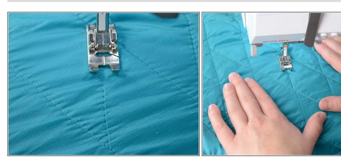
Align the jacket in the sewing machine at a distance of roughly five stitches before the missing stitching.
