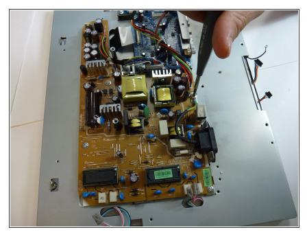
Locate and remove the gold colored 10mm Philips screw located near the black power plug. It holds in a wire that connects to the power plug.
