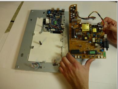
Lift the brown power supply board off of the frame and set it aside.
