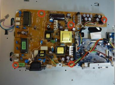
Remove 5 8mm Phillip1 screws, with a Philips 1 screwdriver, located in various places on the board.
