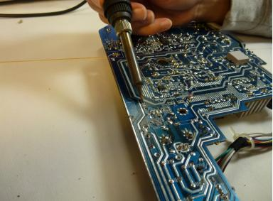
Remove the solder from the three joints attached to the power input.
