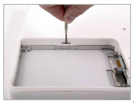
• There is a slot on the wall of the battery compartment that locks the lower case in place. Use a small flathead screwdriver to pry out the slot's lower rim and pull up on the lower case to free the slot from the tabs holding it.
