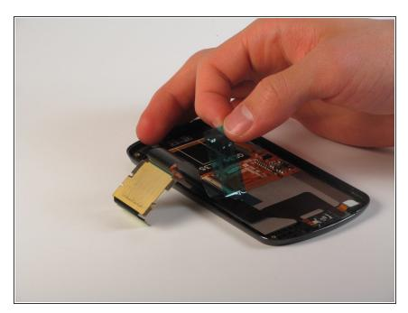
Carefully peel the blue tape from the bottom of the flex cable and set it aside.
