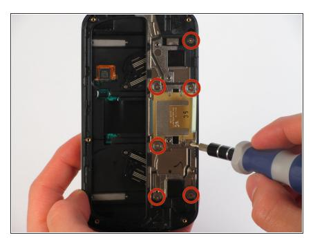
Remove the 7 silver 2mm screws attaching the silver metal plate to the rear panel with the Phillips #000 Screwdriver.
