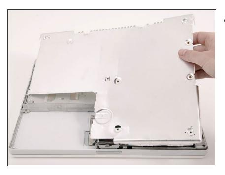
Lift the bottom shield off.
