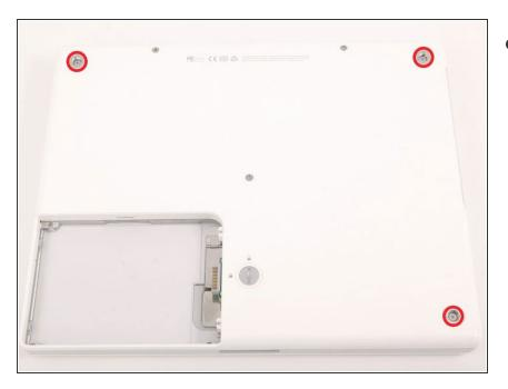
Remove the three newly-revealed Phillips screws.
