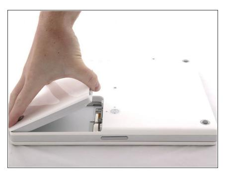
Lift the battery out of the computer.
