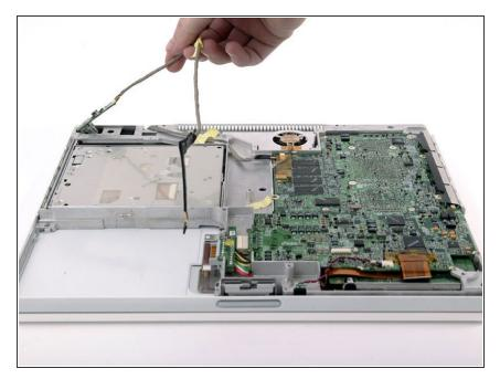
Deroute the cable from around the optical drive, removing tape as necessary, and angle the DC-In board out of its compartment.
