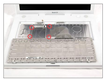
Remove the four silver Phillips screws that secure the RAM shield.
