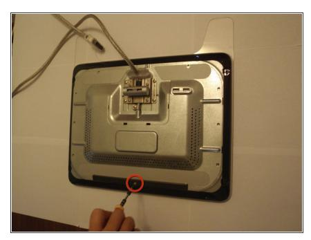
Remove the phillips head screw holding the back panel spacer with the phillips head screwdriver.
