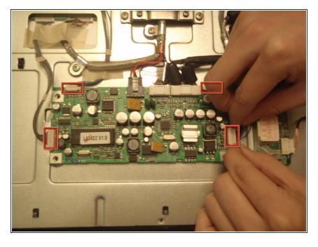
Remove the four braided connections simply by pushing the side of the connectors in and pull out.
