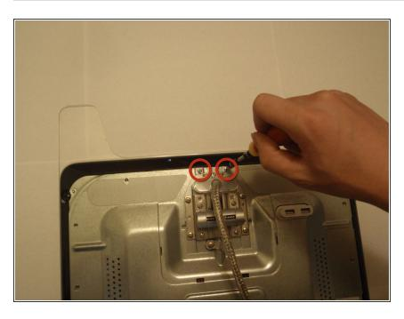
Remove the two phillips head screws near the cable attachment with the phillips head screwdriver.
