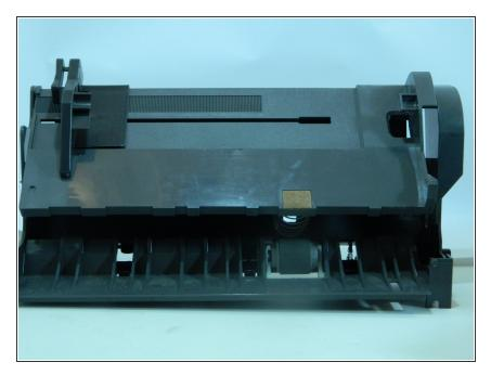
Gently remove the feeder from its place and set it aside from the printer.
