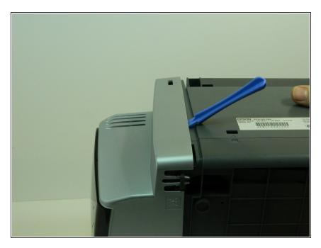
Wedge a blue plastic separator between the plastic housing and the rest of the right panel and push the panel out from the inside to free it.
