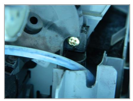
Once you've turned the printer around so the back is faced towards you, locate the screw at the bottom left-hand corner of the paper feeder and unscrew it with a Phillips #1 screwdriver.
