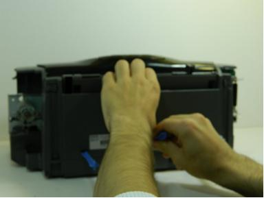
Push on each notch until the retaining tabs are separated from the back plastic cover.
