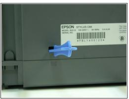
Turn the printer around so the front is facing away. Use three wide-tip blue plastic opening tools and place them inside the notches on the back panel of the printer.
