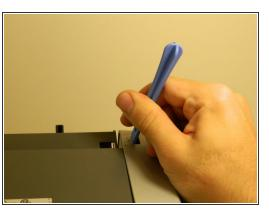
Wedge a wide-tipped blue plastic opening tool inside the gray tab on the upper left-hand corner of the right panel, next to the arrow.
