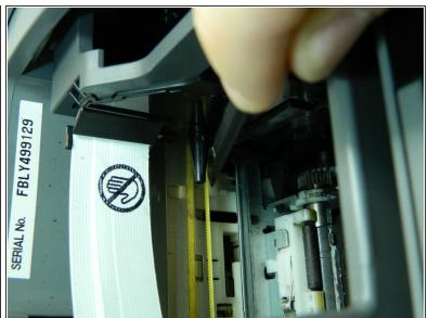
Use the flat end of the spudger to push the white button next to the ink cartridge carrier.
