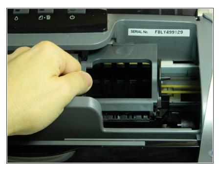
Gently slide the ink cartridge carrier by hand to the left to gain access to the inside of the left panel.
