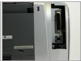
Wedge the flat end of the spudger between the top of the "Parallel" cover and the right panel, and gently pry the upper edge cover away. Completely remove the cover by hand if necessary. The Parallel and USB ports should be exposed.
