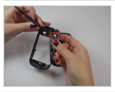
While applying pressure, use your tweezers to remove the screen from the inner casing.
