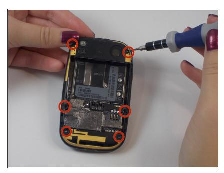
Using the 1.5mm hex screwdriver, remove the 6 hex screws from the inner-most casing.
