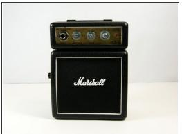
Remove the volume, tone and power knobs by pulling them straight away from the front of the device. If they do not come off easily use the wedge tool to pry them up.
