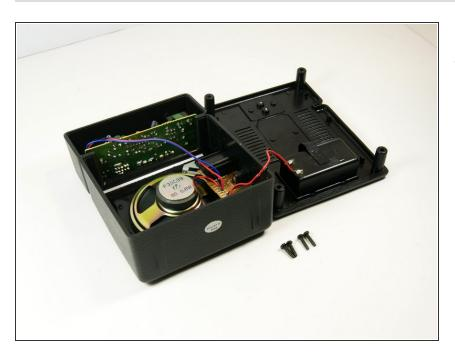
Now pull the back panel off and place it down as shown. Pull the panel straight up so you do not lose the screws.
