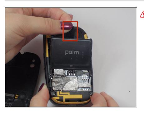
Remove the battery by pulling out the little tab.
