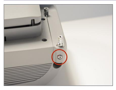
Locate the screw on the back of the radio, in the right hand corner Remove the screw holding the antenna in place.
