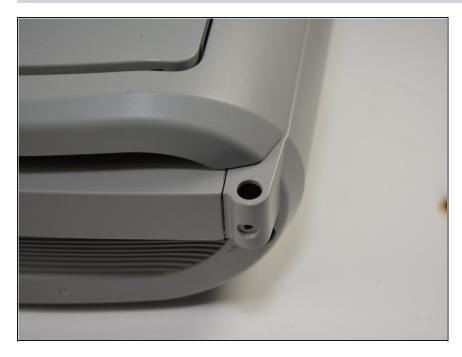
• After removing the screw, pull the antenna straight up and out of the radio.
