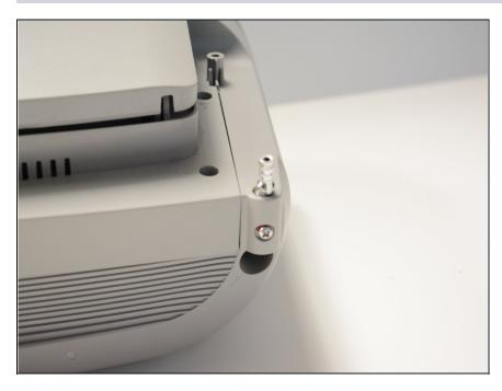
• Insert the new antenna into place. Replace the screw, and attach the antenna to the radio.
