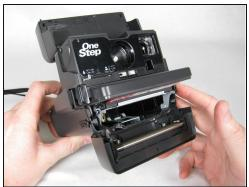
• Fully open the battery/ cartridge compartment by sliding the side tab toward you.
