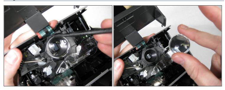
• Carefully use spudger to release lens, then lift lens out of camera with fingers.
