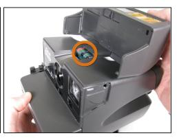
• Separate the flash section of the camera from the main body by unhooking the sides with the spudger.
