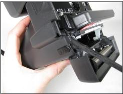
• Insert spudger in between face of camera and sides where the four tabs are located.
