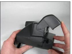
• Open the flash compartment of the camera so it makes a 30 degree angle with the horizontal.
