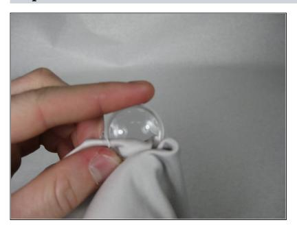
Clean old lens with a microfiber cloth or get a new lens to put back into the camera.
