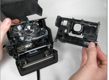
• Once tabs are released, pull face of camera straight out.
