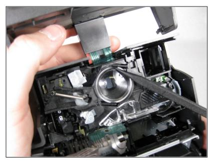
Use spudger to twist the notch on the lens into the opening to remove it.
