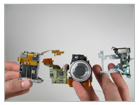
• The remaining pieces from left to right are: the battery casing, zoom lens and flash assembly.
