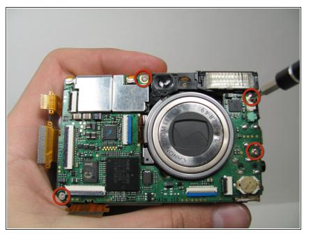
• Unscrew the four Phillips screws using a #0 Phillips screwdriver.
