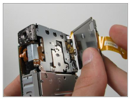
• Lift the LCD away from the rest of the camera.
