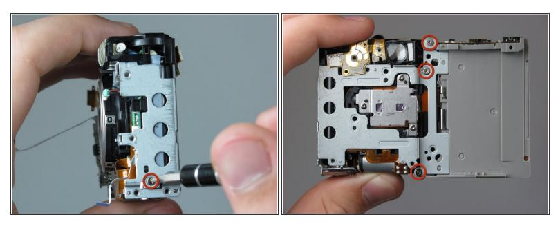
Unscrew one Phillips screws from the side and three Phillips screws from the back panel using a #0 Phillips screwdriver.
