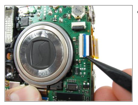
• Lift the blue ribbon gate using the Spudger.
