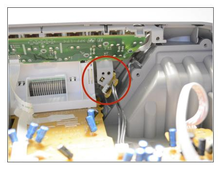
Pull out the audio in jack which is located on the right side of the radio directly below where the buttons are.
