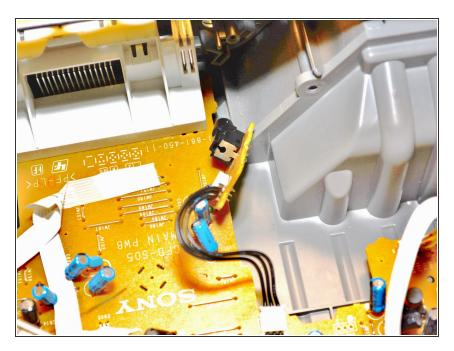
Remove the audio in jack from the circuit board by pulling on the wires where they are connected to the board.
