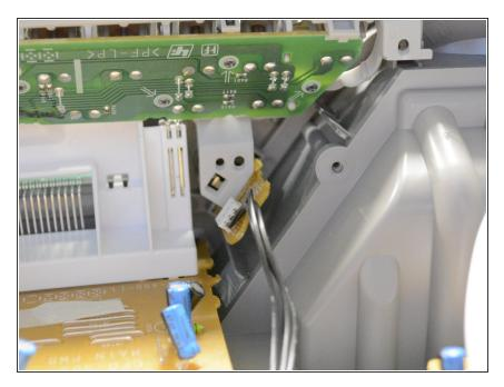
Insert the new audio in jack into the hole on the back side of the front face of the radio.
