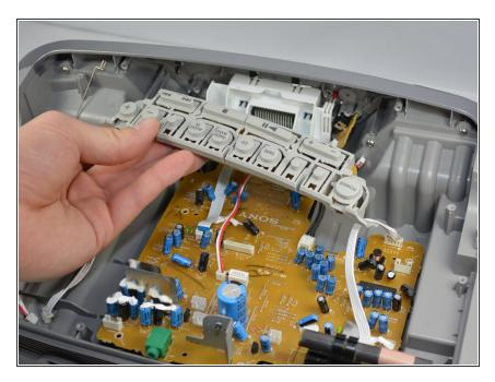
Pull out the buttons of the radio from the inside.
