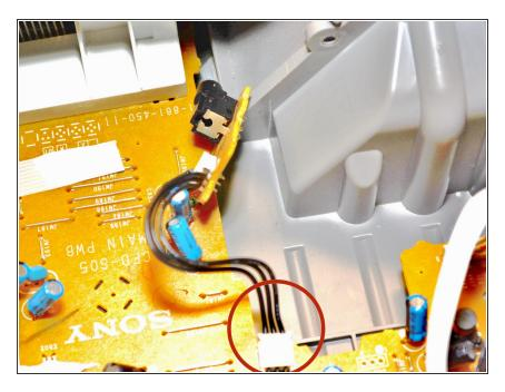
Connect the new audio in jack wires to the circuit board where the old one used to be.
