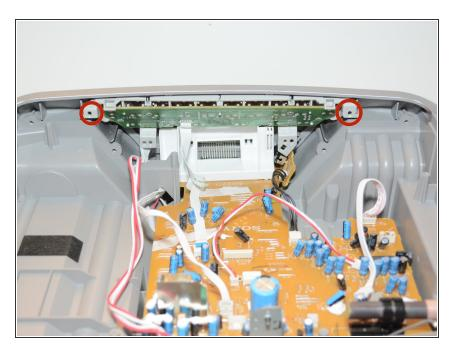
Unscrew the screws on the top right and top left of the back side of the buttons of the radio.
