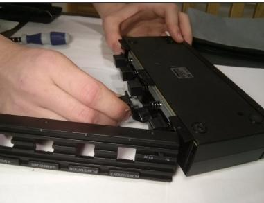
Pull firmly on the button in need of replacement to free it from its housing.
