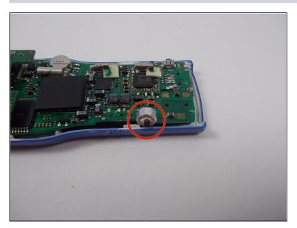
Replace the faulty microphone with a new one in working order.
