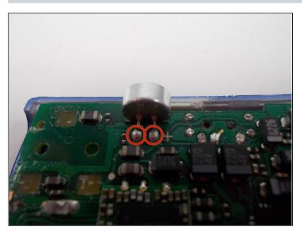
Find where microphone is connected to motherboard via solder.
