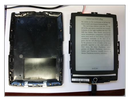
In this picture, you can see the peripheral slots on the back shell where the spurs of the cover are clipped.
