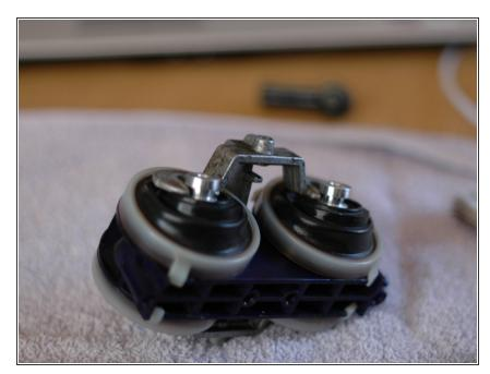
Re-install the metal connector on the metal portion of each diaphragm.
