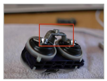
Now that the actuator is out of the door, you're ready to begin replacing the diaphragms. Remove the metal cross-piece between the two sets of diaphragms by gently prying the round metal portion of each diaphragm with a flat blade screwdriver.
