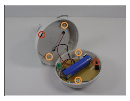
Be careful assembling the device to ensure that the wires do not get caught. Make sure that the switch is lined up with the rubber button and that the screws are lined up with the stand-offs.
