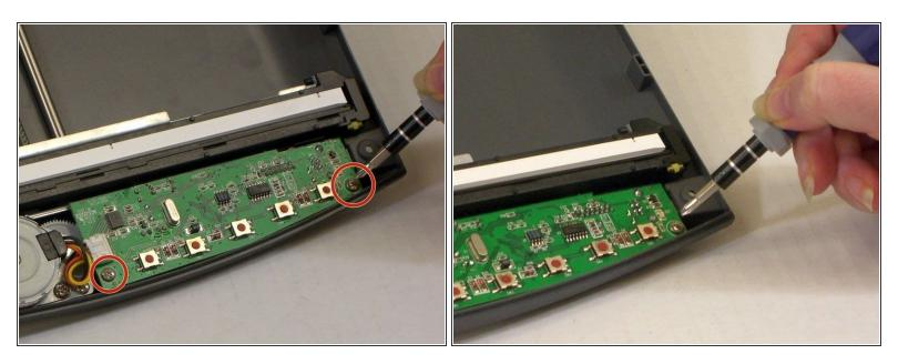
• On the bottom half of the casing, remove the two screws in the motherboard.
