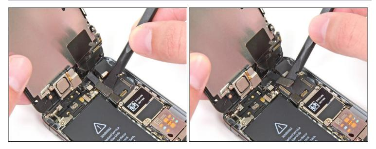
• Finally, disconnect the digitizer cable connector.
