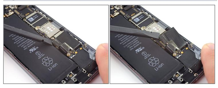
• Use a spudger to pry the Lightning connector cable up from its socket on the logic board.
