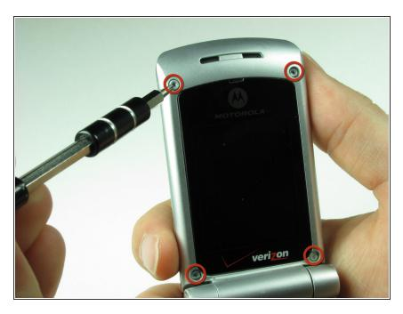
Remove the four Torx-6 screws from underneath the rubber pieces.
