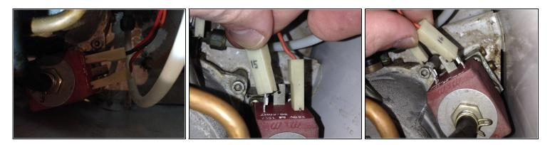
• At the magnetic valve next to the big round boiler, there are two more connectors to label and pull off.
