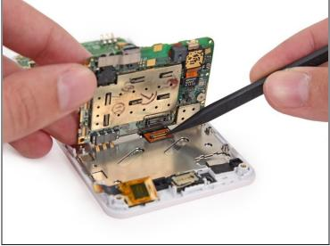
• Use the tip of a spudger to disconnect the display data cable from the back of the motherboard.
