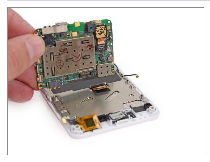
• Remove the motherboard from the display assembly.
