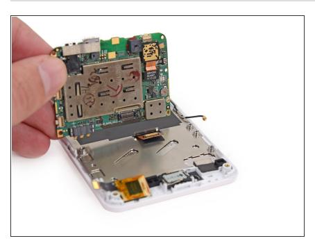
Remove the motherboard from the display assembly.
