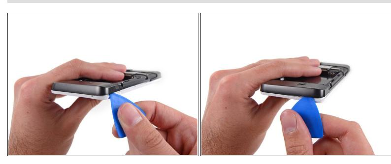
Carefully round the corner, separating the midframe from the display assembly.
