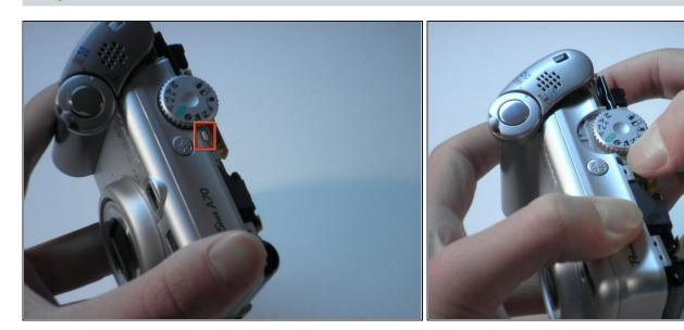
With your right thumb, pull back on the tab while using your left hand to pull the face of the camera away from the body.
