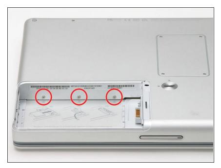
Remove the three small Phillips screws from within the battery compartment.
