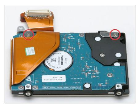
Remove the two Phillips screws on the bottom of the hard drive.
