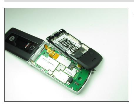
The casing can be easily removed exposing the bottom logic board.
