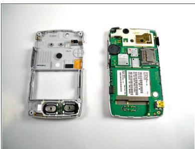
Gently lift and remove the back casing.
