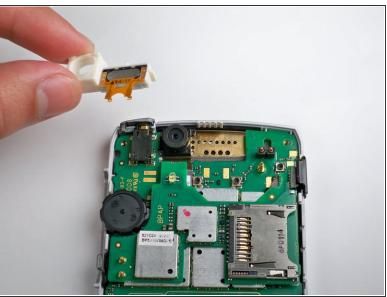
Using your fingers, remove the plastic piece that holds the camera in place.
