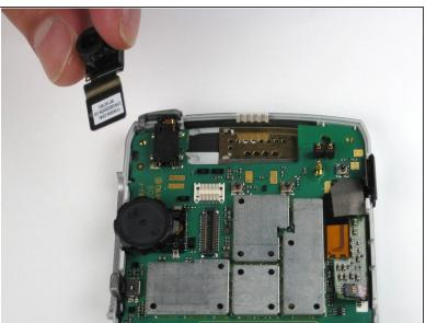
Take out the camera and attached chip with the iPod removal tool. Carefully pry the chip off its connection and the camera will come out too.
