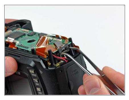
Use a pair of tweezers to pull the USB connector bracket away from the edge of the memory compression board.
