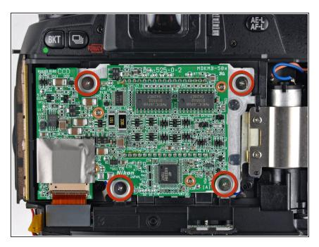
Remove the four 4.8 mm Phillips screws securing the CCD board to the D70.
