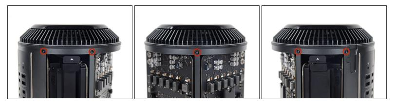
• Remove five 5.1 mm T10 Torx screws from around the outer perimeter of the fan assembly.
