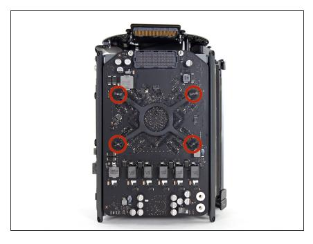
Remove the four 8.4 mm T10 screws from the GPU heat sink bracket.
