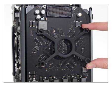
• Remove the GPU heat sink bracket.
