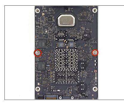
Remove the two 9 mm silver T10 Torx screws securing the IO Board to the IO shield.
