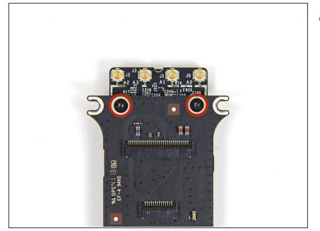
Remove the two 3.7 mm T4 Torx screws securing the AirPort card to the AirPort board.
