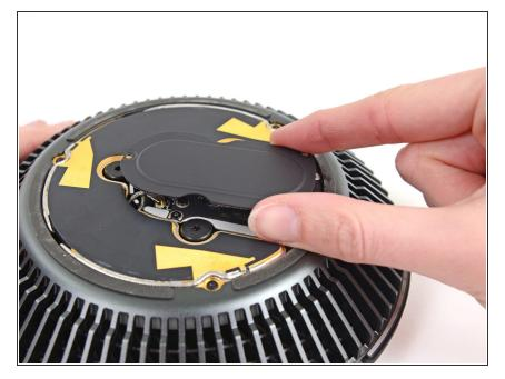
• Lift and remove the metal cover from the AirPort board bay.
