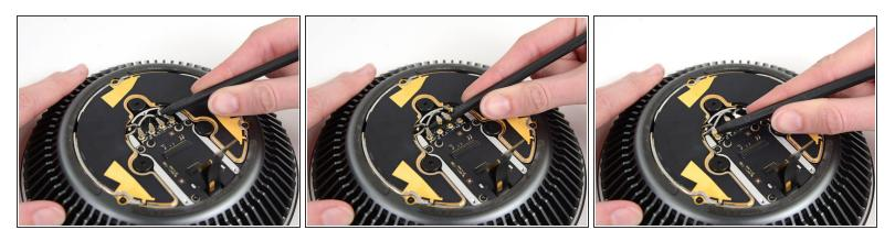
• Use the tip of a spudger to disconnect the four AirPort antenna cables from the AirPort card.
