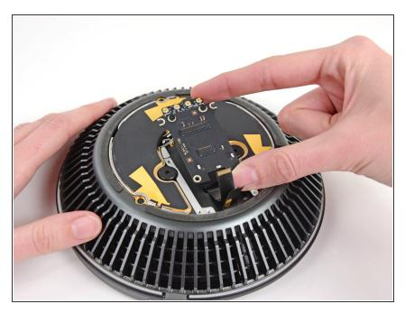
• Remove the AirPort board and card from the fan assembly.
