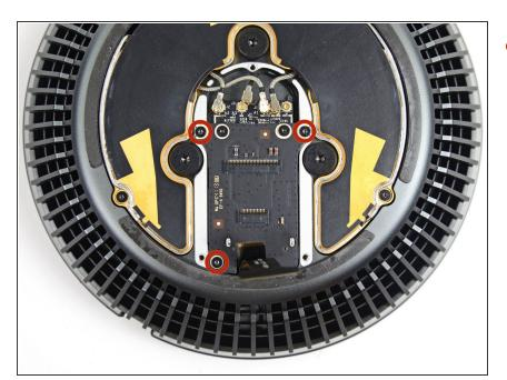
Remove three 3.7 mm T4 screws securing the AirPort board to the fan assembly.
