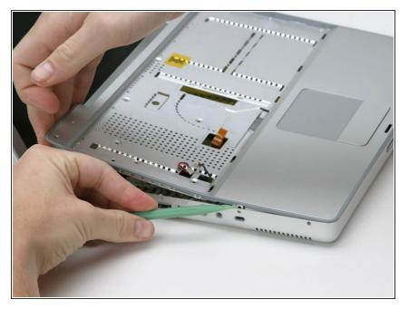
Starting at one of the upper corners near the screen, work around the frame, separating the upper case from the lower case.
