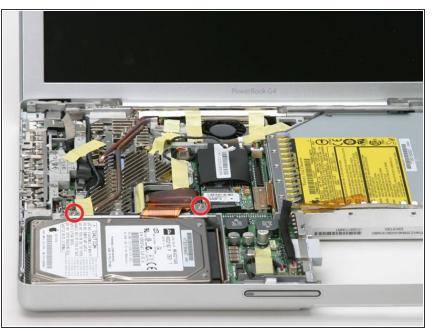
• Remove the two Phillips screws from the hard drive bracket.
