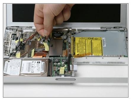
• Disconnect the fan cable from the logic board.
