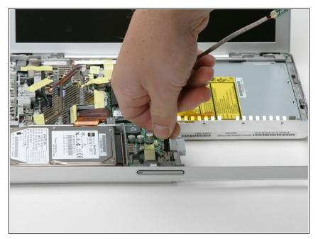
• Disconnect the reed switch cable from the DC-to-DC board.
