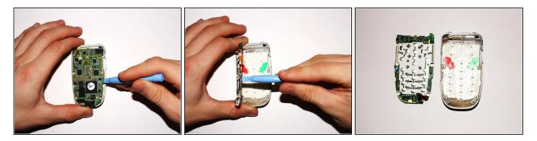
• Remove the green logic board from the phone by gently lifting it up with the plastic opening tool. Be cautious to not break the logic board.
