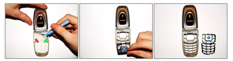
• Remove the keypad from the body by grasping the white rubbery pad and lifting it off the phone.
