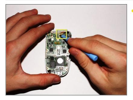
Carefully lift the highlighted connector between the logic board and the screen by using either your fingers or a plastic opening tool as shown in the picture.
