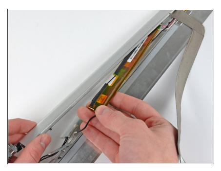
Remove the display inverter assembly from its recess in the clutch cover.
