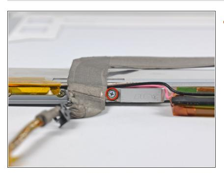
Remove the single 2.5 mm Phillips screw securing the display data cable to the front display bezel.
