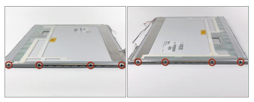
Remove the four black 3.2 mm Phillips screws from both sides of the display (eight screws total).
