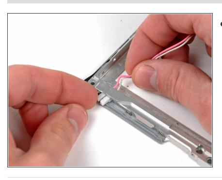
With the LCD partially removed from the front bezel, carefully push the backlight connector through its tunnel in the front bezel.
