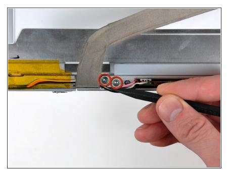
Remove the two 10.3 mm T8 Torx screws securing the left side of the clutch hinges to the front bezel.
