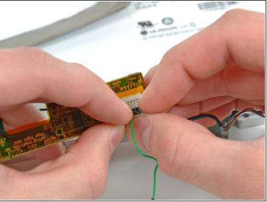
• Carefully grasp the inverter connector with the ends of your fingertips and pull it straight down.
