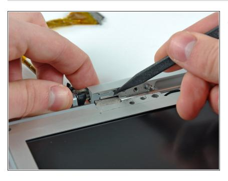
Use the tip of a spudger to remove the plastic end cap from the right side of the clutch hinges.
