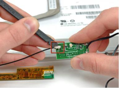
Use the flat end of a spudger to pry the the antenna cables straight up off their sockets.
