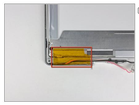
If necessary, remove the piece of tape covering the inverter lead.
