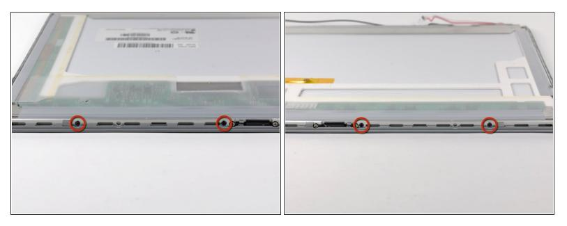
• Remove the four black 3.2 mm Phillips screws from the top side of the display.
