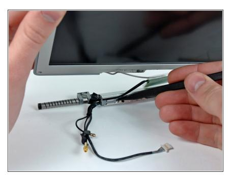
Use the tip of a spudger to pop the plastic end cap off the left side of the clutch cover.
