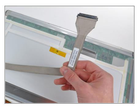
Remove the display data cable from the LCD assembly.
