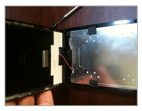
As you can see here, the back edge where the light is has a small connector to the rest of the board. this pulls out easily.
