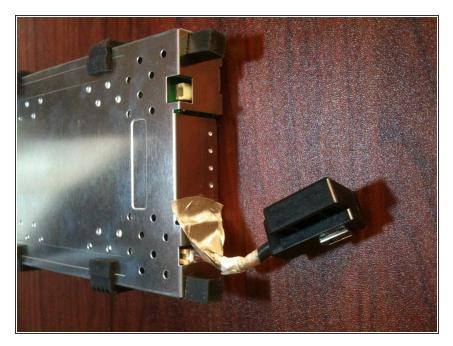
The bottom casing lets the drive fall out and you have two metal shielding pieces holding the drive in place with four rubber bumpers. The USB dongle is held in place with tape, but it's easily pulled up and removed from the plug.
