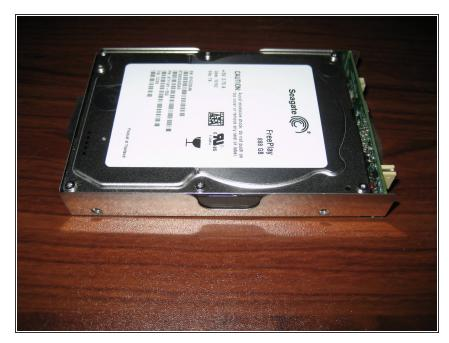
The top cover slides backwards, away from the board to allow access to the 888GB drive. The drive pulls out from here and easily disconnects from the controller board.
