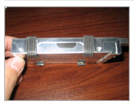
• After the USB dongle is removed, there are four phillips screws on the sides that hold the two metal pieces in place. Once those are removed, the rubber bumpers are easily removed as they are only held in place by the cement as well.
