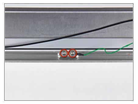
Remove the two 10.3 mm T8 Torx screws securing the center of the clutch hinges to the front bezel.
