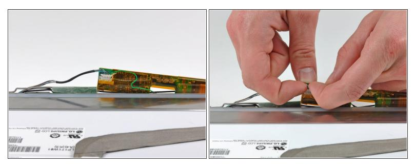
Use your fingernails to pull the ears on both sides of the inverter cable connector away from its socket on the inverter board.
