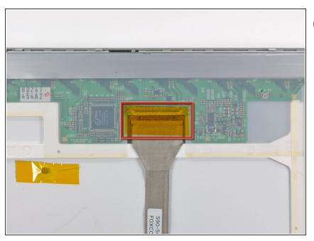
*i* If present, remove the piece of tape covering the display data cable.
