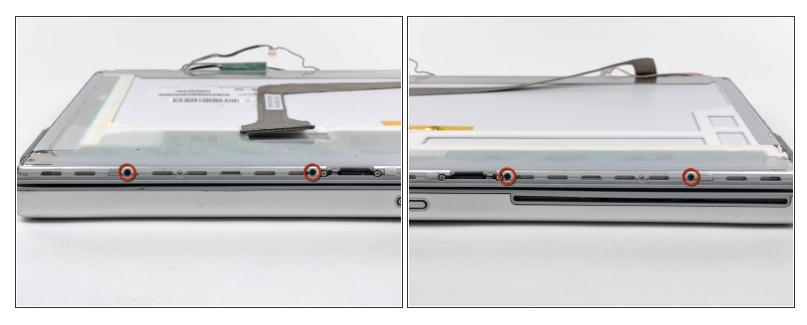
• Remove the four 3.2 mm Phillips screws from the top portion of the LCD assembly.
