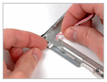
• With the LCD partially removed from the front bezel, carefully push the backlight connector through its tunnel in the front bezel.
