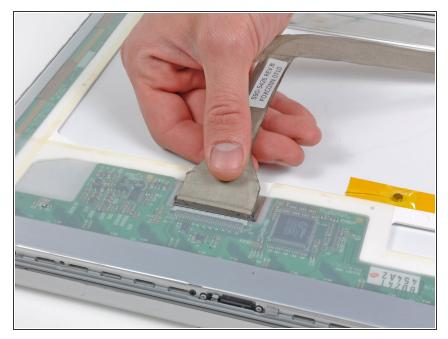
• Pull the display data cable straight away from its socket on the LCD.
