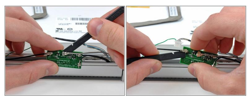
• Use the flat end of a spudger to pry the the antenna cables straight up off their sockets.
