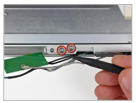
Remove the two 10.3 mm T8 Torx screws securing the right side of the clutch hinges to the front display bezel.
