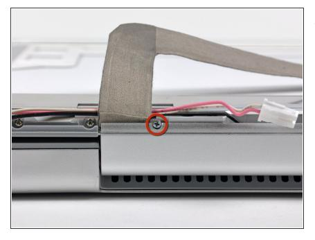
Remove the single 2.5 mm Phillips screw securing the display data cable ground loop to the front display bezel.
