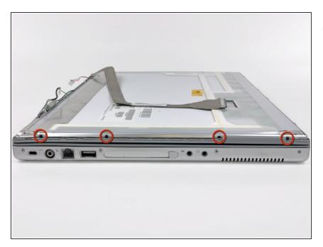
Remove the four 3.2 mm Phillips screws securing the left side of the LCD assembly to the front display bezel.
