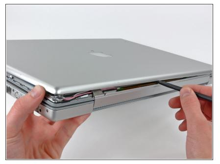
Slightly lift the recently-freed corner of the rear display bezel to separate the clips with a spudger along the span of the clutch hinges.
