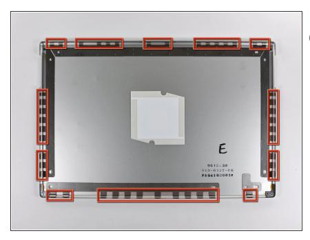
(i) The picture at left (rear panel already removed) shows the locations of the metal clips (shown in red) that snap on to the front display bezel. In the next few steps, you will use a small flathead screwdriver to release these clips from a ridge around the perimeter of the front display bezel.
