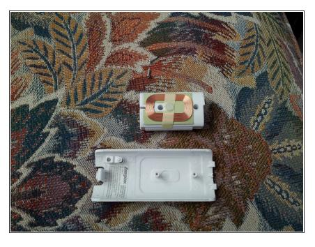
Pull out the battery from the case. It should slide out easily.
