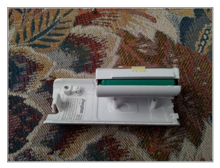
Using your fingernail or a small screwdriver, carefully separate the two halves of the battery casing.
