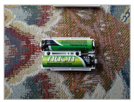
Once the contacts and compartment are clean, insert your new rechargeable batteries.
